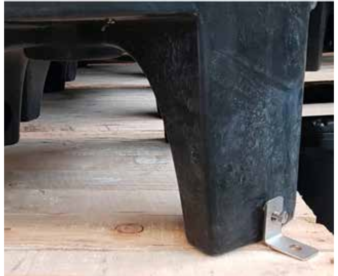
Figure 4 - Bolting the feet
