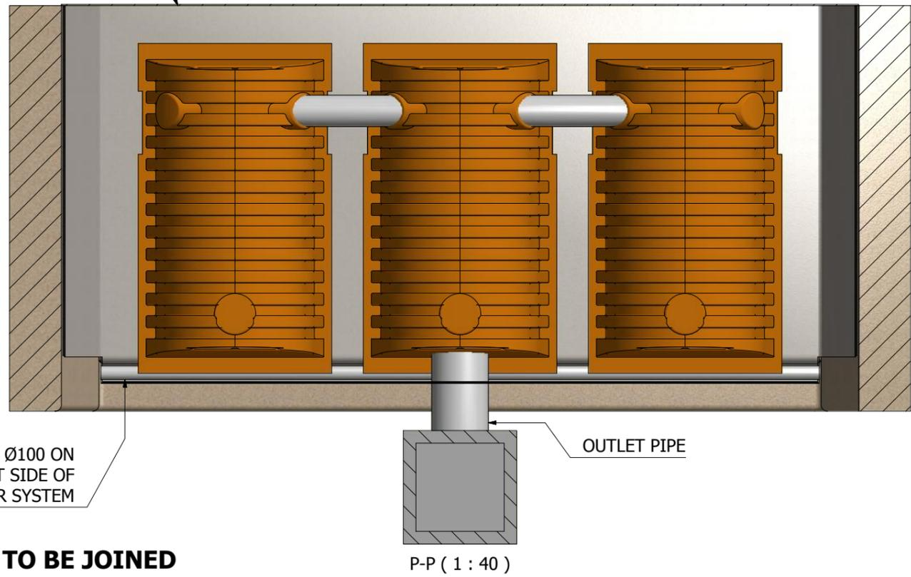
**NOTE: ALL LINER TO BE JOINED IN A WATER TIGHT FASHION & INSPECTED PRIOR TO INSTALLATION.**
