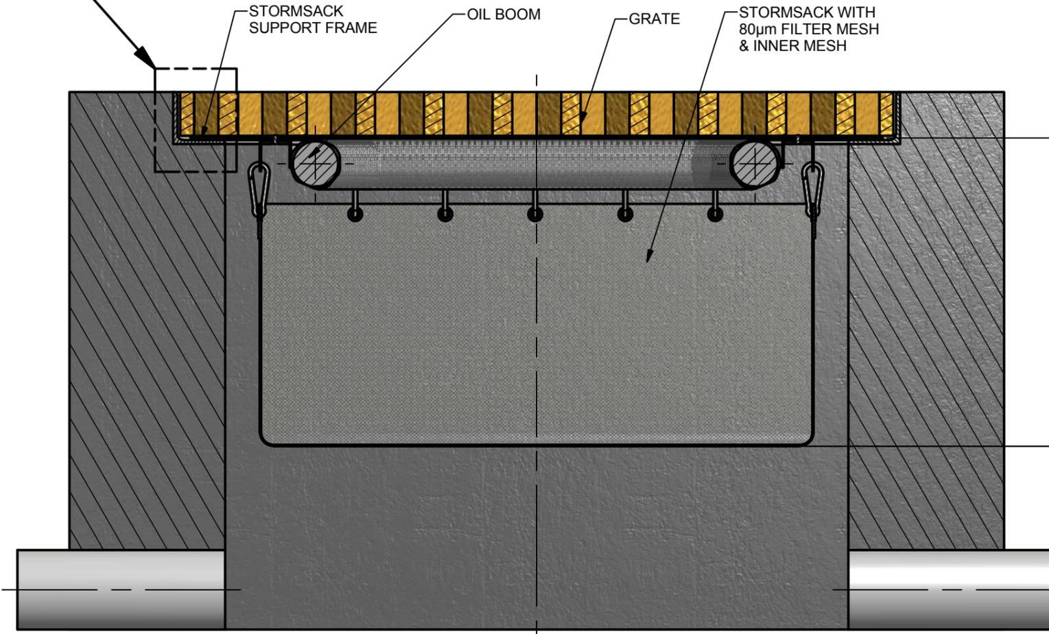
GRATE SUPPORT FRAME STORMSACK SUPPORT FRAME GRATE
